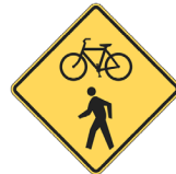
Fig 3.26 MUTCD W11-15 The BICYCLE/PEDESTRIAN WARNING sign (W11-15) may be used as a substitute of the W11-1 where a sidewalk is parallel to the separated bike lane and motorists may not be expecting to cross either the bicycle or pedestrian crossing
